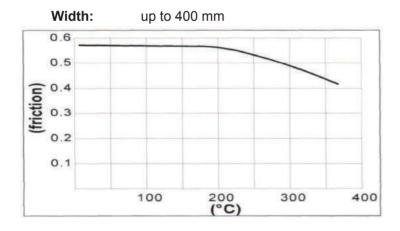
Above information is based on a brake drums made from ST52. Any other material can have a slightly different result.
